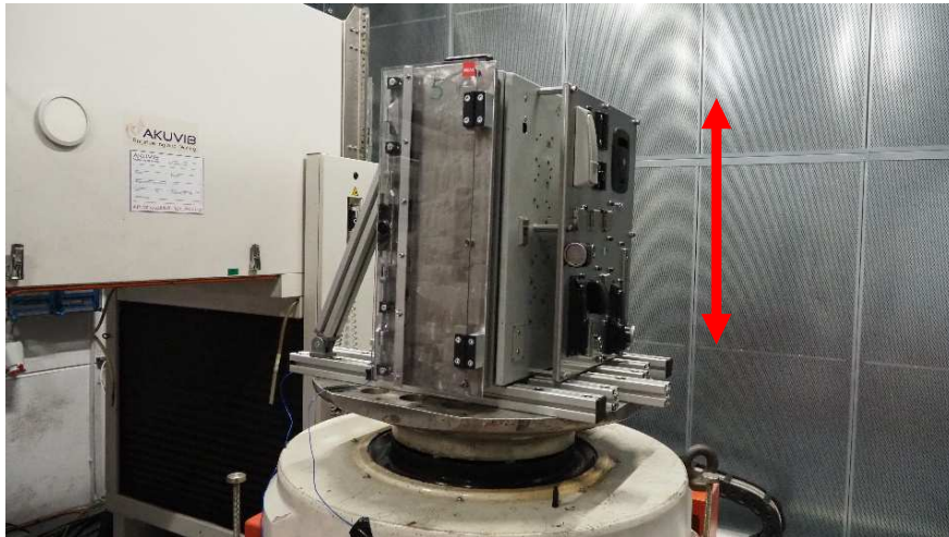
Fig. 1: Specimens during the vibration and shock test in direction vertical
