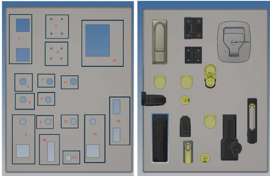
Fig. 5: Arrangement of the specimens (sheet metal 1)
