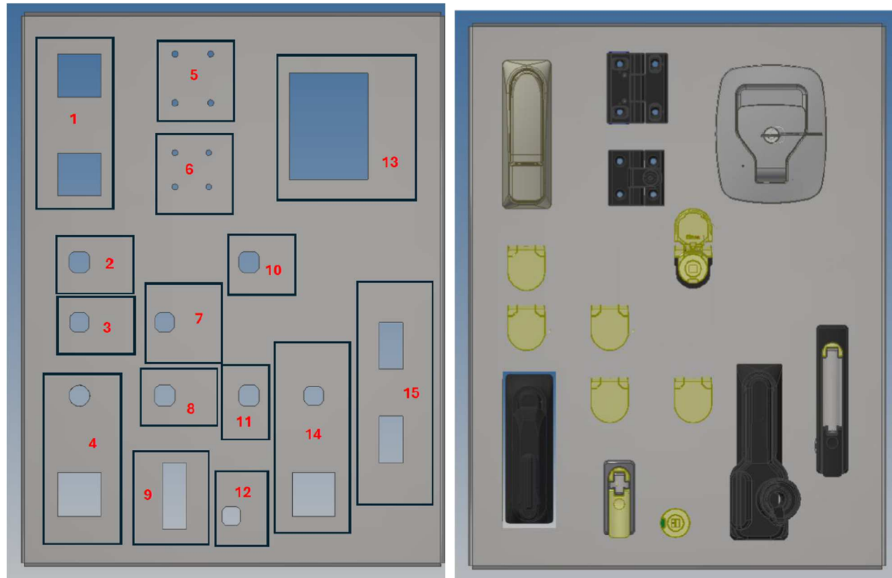
Fig. 7: Arrangement of the specimens (sheet metal 3)
