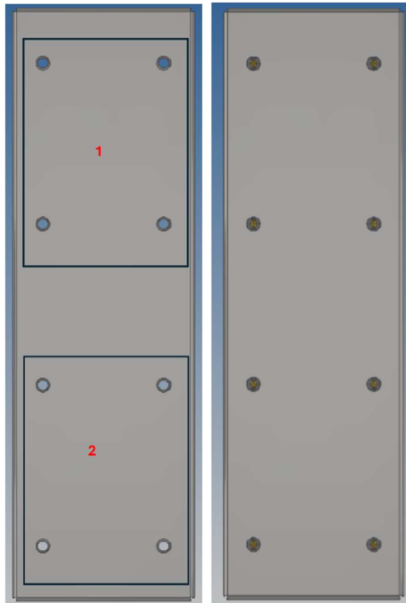
Fig. 8: Arrangement of the specimens (sheet metal 4)
