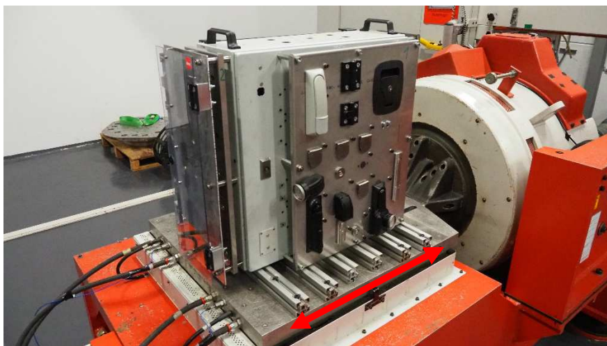
Fig. 2: Specimens during the vibration and shock test in direction horizontal 1
