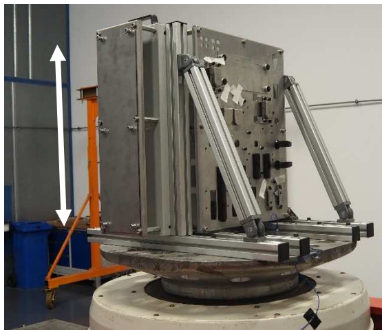
Fig. 3: Specimens during the vibration and shock test in vertical direction
