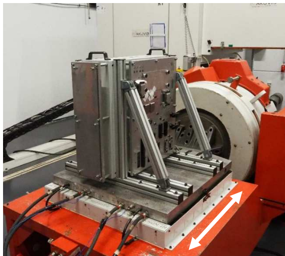
Fig. 1: Specimens during the vibration and shock test in the first horizontal direction
